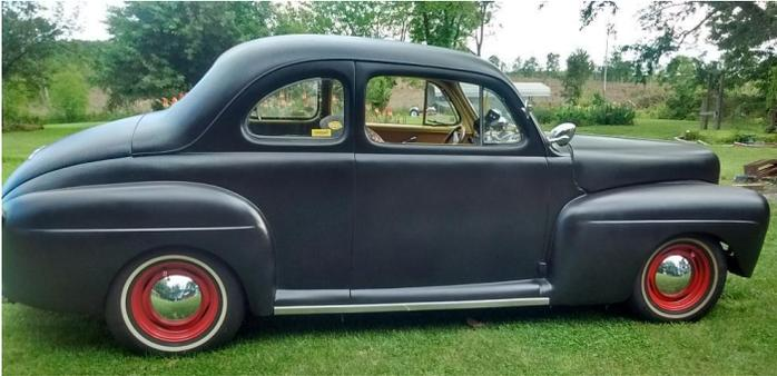
Dummy spots, baby Moons, no front bumper, mostly Oldsmobile running gear, flat black primer paint, fits right into the style of car that we all wanted back-in-the-day. Donnie stated that having owned the car for about ten years it's still a work in progress. Wasn't that true of all hot rods of our youth?
