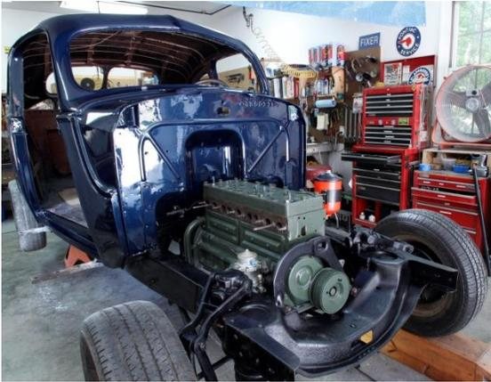
I now installed the radiator and hose connections in preparation for adding the coolant but I will have to wait for the exhaust system to arrive around the 13<sup>th</sup> of September before I can start the engine. There were many other small items that were connected which are too numerous to mention at this time.
