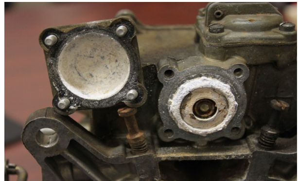
Ethanol damage to a carburetor. Photo by Tom Shaw, courtesy SEMA.
