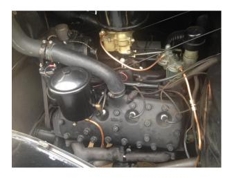
The original 221 CID flathead V8 engine is replaced by a 1948 239 CID V8 Ford. Reggie installed a brand new carburetor and electronic ignition and he stated "... it couldn't have run any better when it was new."
