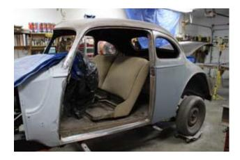
Otto came over and helped me with the paint removal and that has really helped to speed things. We took the front fenders, hood and cowl over to the sand blaster and I now have all of this stuff to repair and prime.
