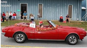
The Firebird was purchased by Donnie over thirty-one years ago. It has a matching number 400 CID (6.6L) 4V, Muncie four speed trans, factory Hurst shifter, factory hood tach, factory red-on-red with one repaint, 10.75 compression, and original AM/FM radio.
