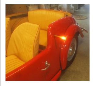
Notice that the seat & top piping matches the car's color. Also notice the "European style side semaphore turn signals" that pop-up and illuminate when actuated for left or right turns.
