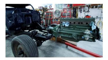
Since then I have fitted many parts together that I could not do with the engine out and I have Patty ready to start except for the exhaust system. I hooked the starter up to the battery and turned the motor over to prime all of the oil galleries in the engine and check for a good oil pressure. This was an exciting moment because it meant I was very close to starting the motor. I also checked the ignition timing to
